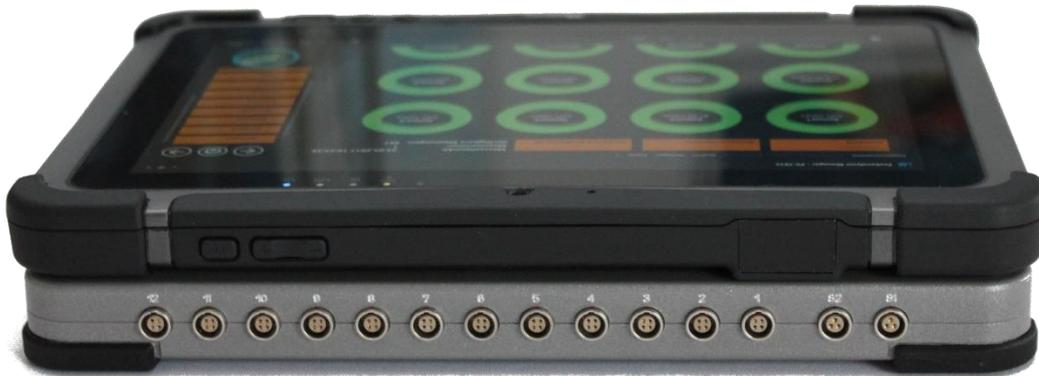
*Picture 3 Sensor connections*
